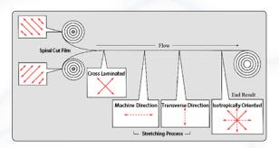
The cross-laminated film has to go through a stretching process in different directions, so the molecules of the final products are isotropically oriented. This process highly enhances the strength of the film.
